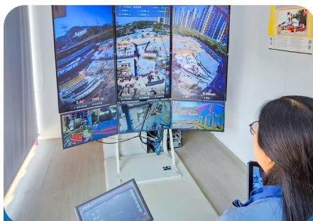
Smart tower crane operations enhance construction safety at Ha Ko Po Tsuen project
