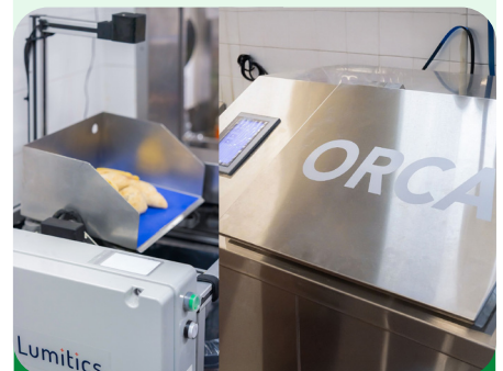
The Lumitics system and ORCA food waste digester analyze food waste patterns through AI technology
