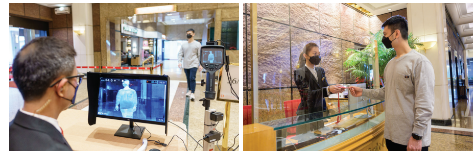
• The infrared temperature-scanning system in the lobby not only helps reducing manpower to conduct temperature checks for the building's users, but also minimizes waiting times
