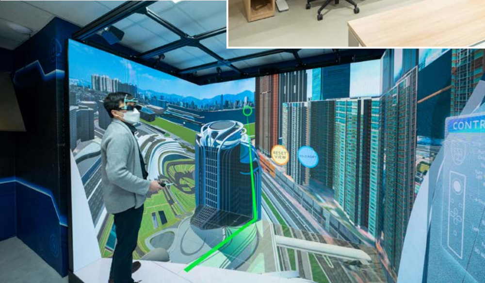
The Group introduces Cave Automatic Virtual Environment (CAVE), utilizing 3D projection screens and motion-sensing devices, making every aspect of project management more precise and effective. 集團引入虛擬實境互動系統 (CAVE)，透過立體投影屏幕和體感操作設備，令項目管理的各環節更加精準便捷。
