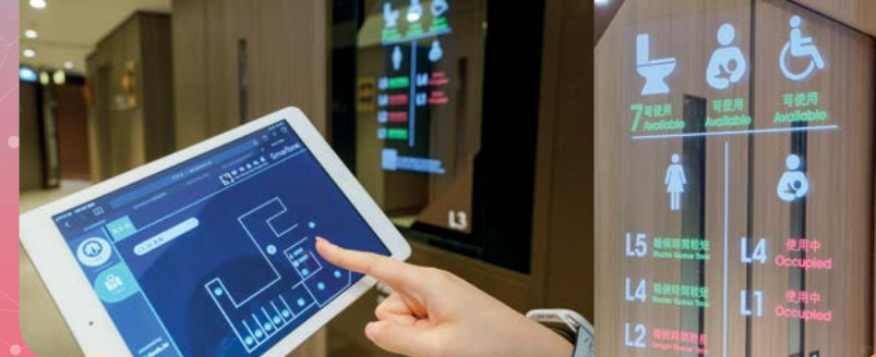
The digital signages at Metroplaza's restroom entrances leverage the 5G network and sensors to show the restroom's real-time occupancy, reducing queuing time 新都會廣場洗手間外設有電子顯示屏，運用5G網絡及感應器，提供洗手間的即時使用情況，有助縮短等候時間
