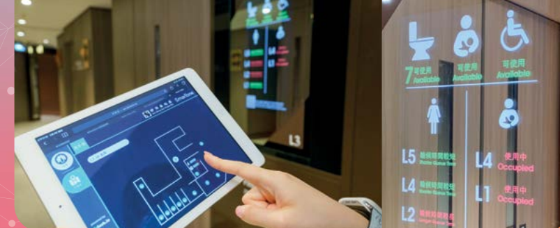
The digital signages at Metroplaza's restroom entrances leverage the 5G network and sensors to show the restroom's real-time occupancy, reducing queuing time 新都会广场洗手间外设有电子显示屏,运用5G网络及传感器,提供洗手间的实时使用情况,有助缩短等候时间
