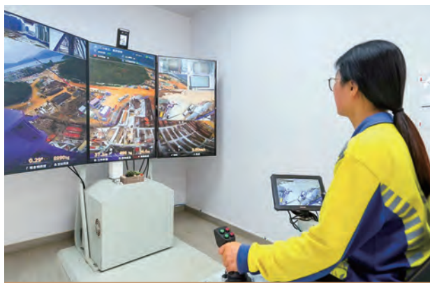
○ Sanfield deploys 5G-enabled unmanned tower cranes across various sites
